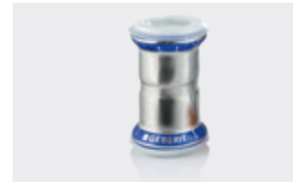
↑ GEBERIT MAPRESS STAINLESS STEEL: PRODUCT MATERIAL 1.4401 Tested and approved for wet and dry sprinkler systems – for example, by VdS and FM – and according to DIN 14462 also suitable and can be used for 'wet', 'wet/dry' and 'dry' extinguishing water pipes.
